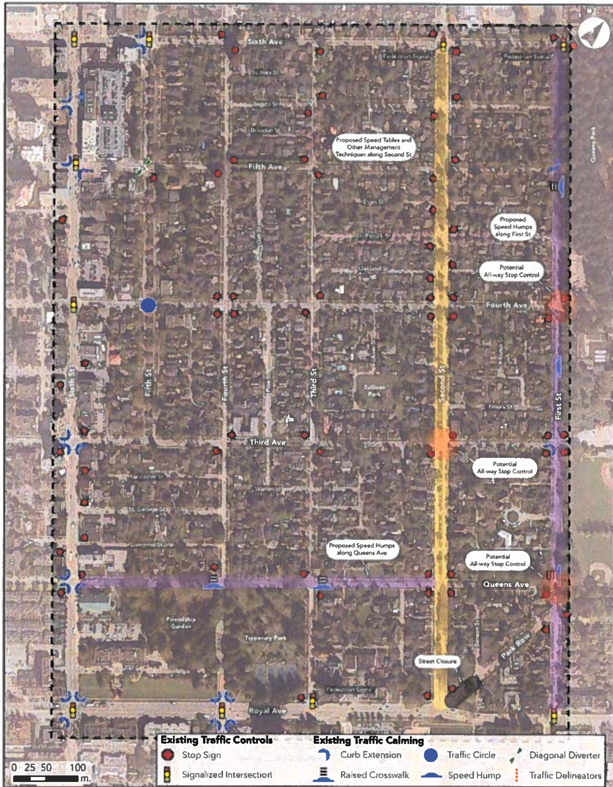
Figure 3: Proposed Traffic Calming Devices and All-Way Stops
