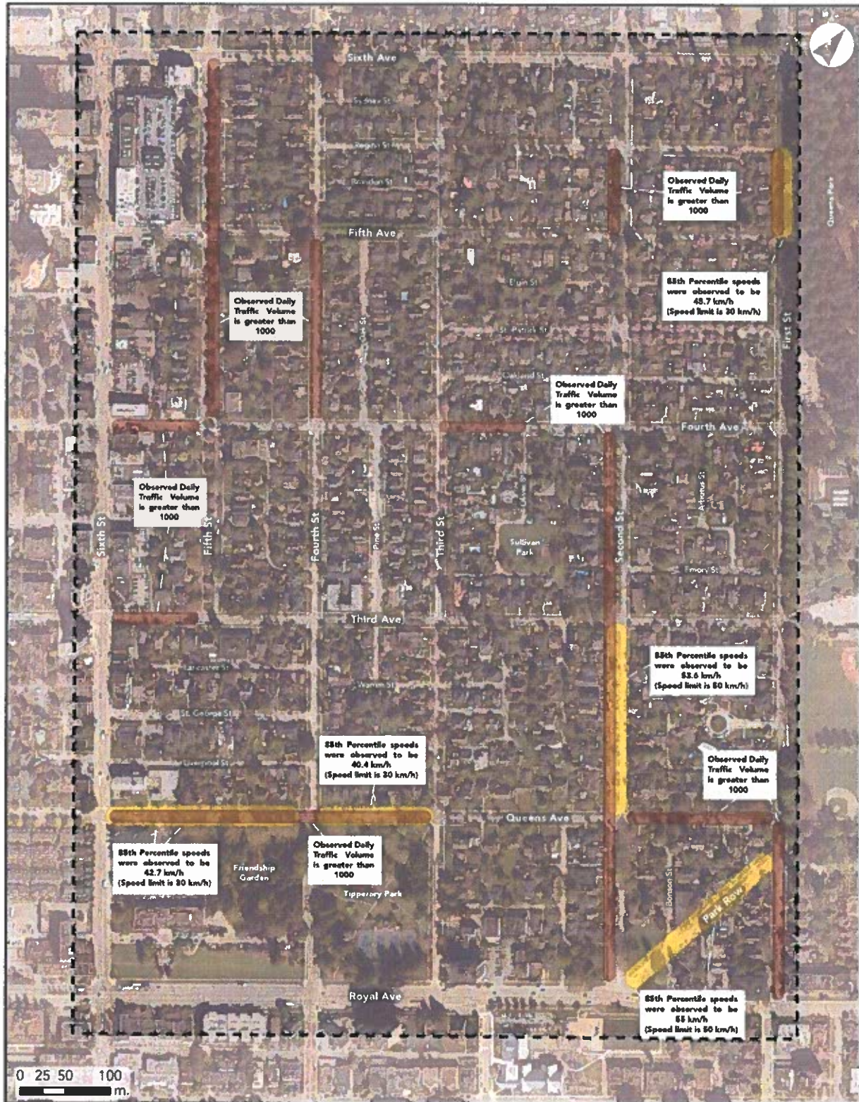
Figure 2: Areas of Concern Identified by Speed & Traffic Volume Data
